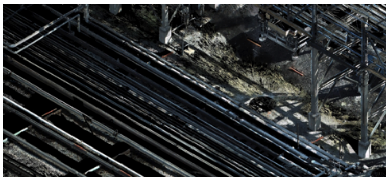
3D Point Cloud Scan of Pipe Alley Prior to Piping Model Creation
