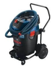
The large capacity Bosch wet/dry extractor has a water-level sensor to help preclude overfilling and a discharge hose for easy drainage. The easy-to-transport unit has sturdy metal castors designed to withstand jobsite terrain, a metal frame with a height-adjustable fold-down push handle for easy maneuverability. The unit features a dumping mechanism for emptying convenience.
